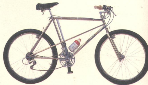
1977 Breezer owned by Charles Kelly. Second Breezer built, equipped with Phil Wood hubs, Magura handlebars and brake levers, Suntour thumbshifters and derailleurs, Weinman cantilever brakes, Campagnolo seatpost with custom modification to accept Brooks B-72 saddle, TA cranks, Cook Brothers fork custom modified by Joe Breeze.
