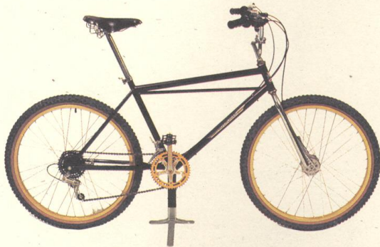
1979 Lawwill-Knight Pro cruiser 5-speed owned by Mert Lawwill. Sturmey-Archer Drum brakes, Tomaselli brake levers, Mert Lawwill custom stem, motorcycle handlebars, SunTour thumbshifter and rear derailleur.
