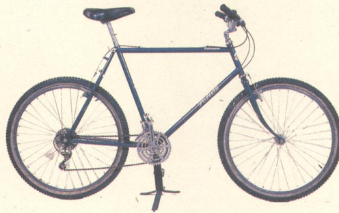
1982 Stumpjumper with TA cranks, Tomaselli brake levers, Mafac cantilever brakes, SunTour derailleurs and thumbshifters. From the Mountain Bike Hall of Fame and Museum.
