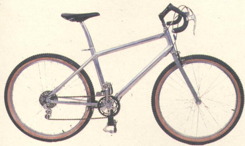
Charlie Cunningham 1979 5-speed with handmade toggle brakes, magnesium stem, titanium chainguide, titanium toe clips, Type II fork, SunTour ARX rear derailleur. From the Mountain Bike Hall of Fame and Museum.
