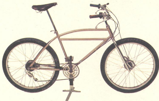
Schwinn Excelsior circa 1935 built and owned by Gary Fisher and used to set the Repack course record of 4:22. Equipped with Union front and Worksman rear drum brake, Honda motorcycle brake levers, Campagnolo seatpost quick release, SunTour thumbshifters, Shimano 600 rear derailleur, SunTour Spirt front derailleur, TA cranks.
