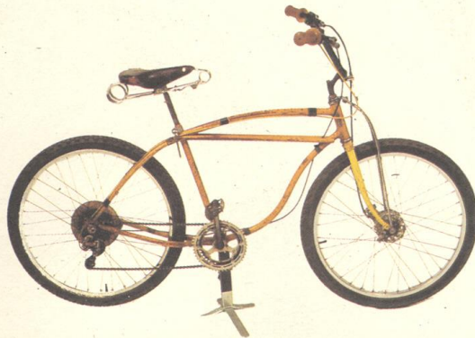
1950 Schwinn Spitfire modified by Gary Fisher in 1976 for Al Strong and sold to Bob Burrowes. Used by Burrowes to win the first Repack race in the fall of 1976. Features drum brakes front and rear, extra-long 7" cranks, Schwinn fork brace, BMX high-rise handlebars, Suntour thumbshifter, seatpost quick release from Schwinn Exercycle.
